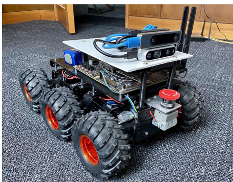
Fig. 10 Rover robot used in real-world transfer. The policy model is trained on simulator and deployed on the real robot. It is equipped with an IMU as well as an RGB-D module
