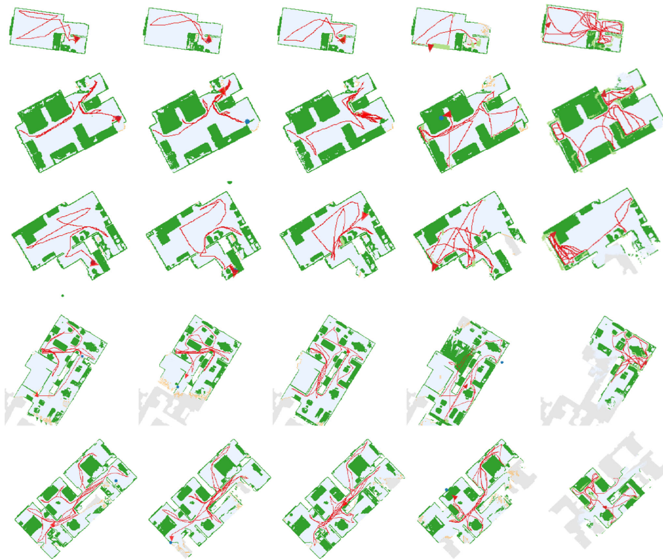
Fig. 13 Trajectories of different methods after 1000 time steps. From left to right columns: our approach, look-around option disabled, frontier method, arbitrary point method and atomic action method. Each row represents a selected scene. Green areas represent obstacles, while light blue represents free space. Red lines indicated the trajectories of agent. Orange dots are the frontiers. Unexplored areas are in gray. We
